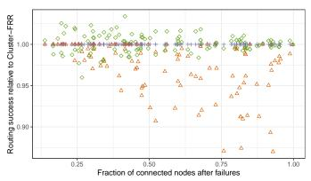
Fig. 6. Relative routing success rates of algorithms on the Topology Zoo dataset, for all graphs containing between 20 and 50 nodes, as a function of the fraction of nodes remaining connected to the destination after 10 RANDOM failures, compared to Cluster-FRR.
