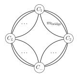
Fig. 2. Illustration of the ring-of-cliques network topology model. Each of the cliques  $C_1, C_2, \ldots, C_L$  has an internal link connectivity  $k_{\rm clique}$  and there are  $m_{\rm bridge}$  links between adjacent cliques.
