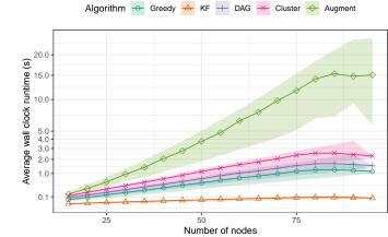
Fig. 7. Average wall clock times for the precomputation of the routing tables of each algorithm on networks of increasing number of nodes. The shaded area symbolizes the 10 and 90 percentiles of the distribution sampled over 80 independent runs. The y-axis is square-rooted.
