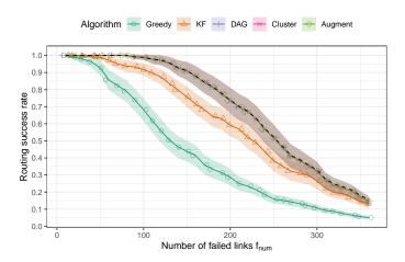
Fig. 3. Routing success rates on the ring of cliques for varying number of RANDOM failures and for different algorithms. The black dashed line represents the average value of  $\rho$ , the percentage of the number of nodes in the connected component containing the destination (after failures), and is therefore a statistical upper bound on the success rate. Ribbons represent 1/4th of the standard deviation over 200 independent repetitions.
