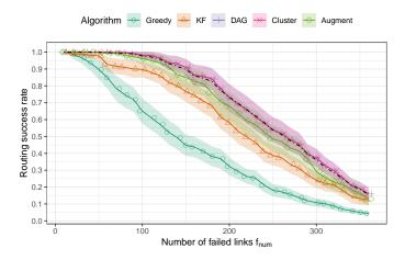
Fig. 4. Routing success rates on the ring of cliques for varying number of CLUSTER failures and for different algorithms. The black dashed line represents the average value of  $\rho$ , the percentage of the number of nodes in the connected component containing the destination (after failures), and is therefore a statistical upper bound on the success rate. Ribbons represent 1/4th of the standard deviation over 200 independent repetitions.
